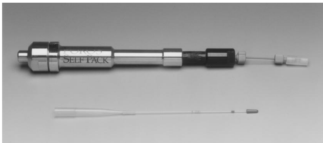
FIG. 2. Column packing devices. The Poros Self-Pack reservoir (top) is shown with a PEEK column used as an adapter and with a column attached ready for packing. The dry-packing assembly (bottom) is shown with the capillary tube (125 mm) connected to the pipet tip with a small section of silicone tubing and sealed with a 1/16-in. tubing cap.
